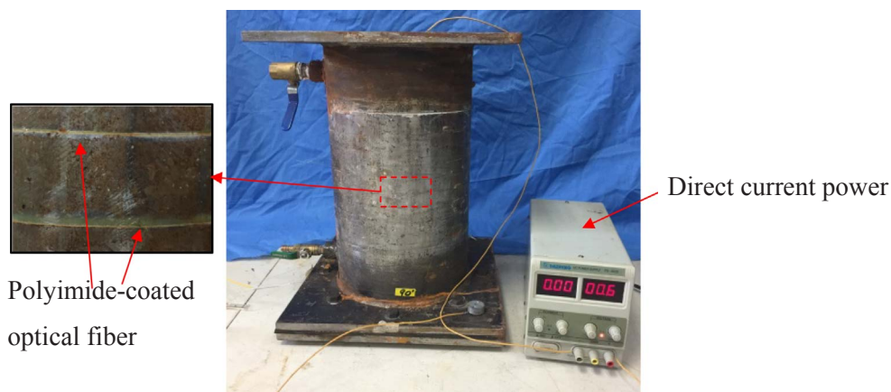
Fig. 4. Corrosion test pipe and direct current power.
